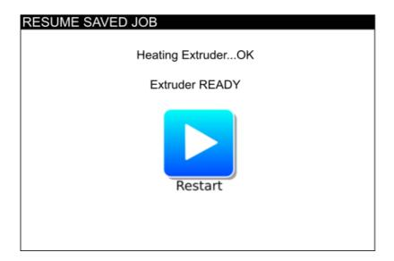
Now the printer start to extrude slowly (this to be sure that the nozzle is not empty of material). Tap the display to restart the printing job.
