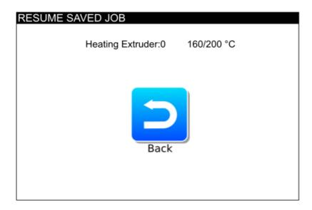
When temperatures have reached the target, the display show the following:
