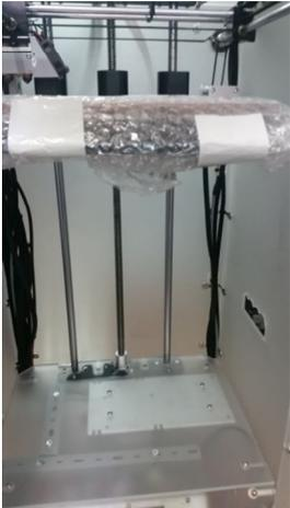
9: remove the four (4) blue tape pieces located at the corners of the bed
